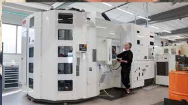
One of our two Yasda Px30i machines, a 5-axis precision machine with integrated automation.
