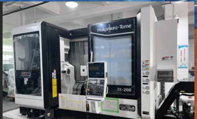
Our latest investment in 2024: a multi-operation lathe with a B-axis, turret, and bar feeder.
